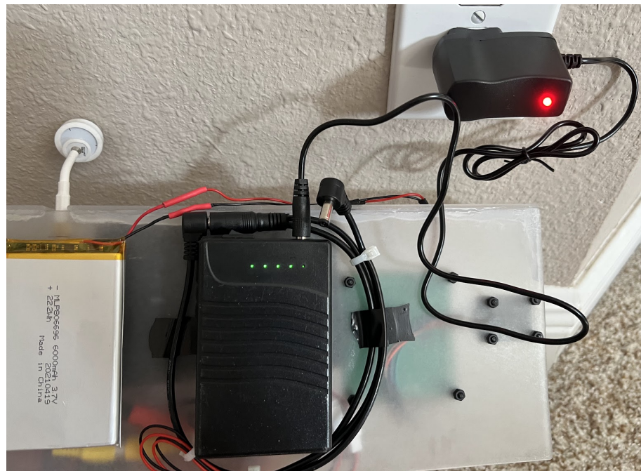
Figure 41: 11.1V RCS Charger Operation
