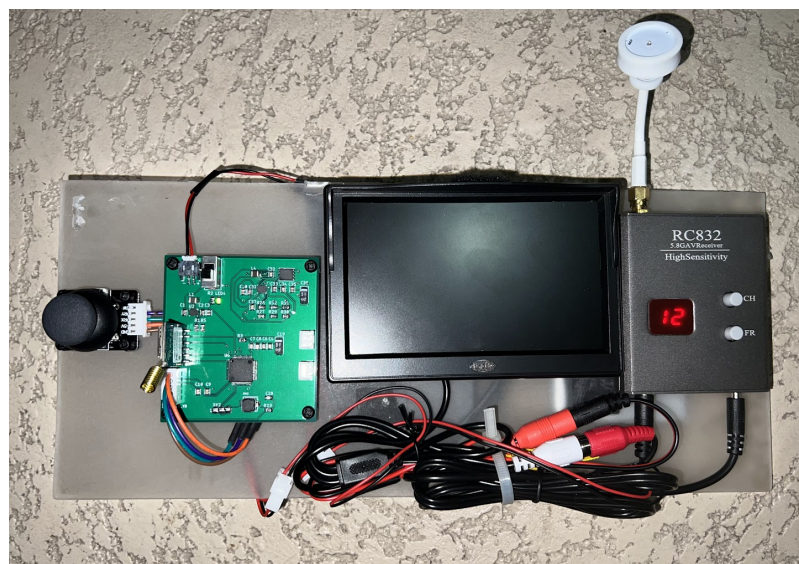
Figure 37: Top View of the Rover Control Station
